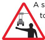
A signal person must be on hand to assist the operator whenever the equipment is near overhead power lines.
